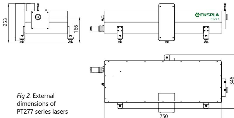
Fig 2. External dimensions of PT277 series lasers
