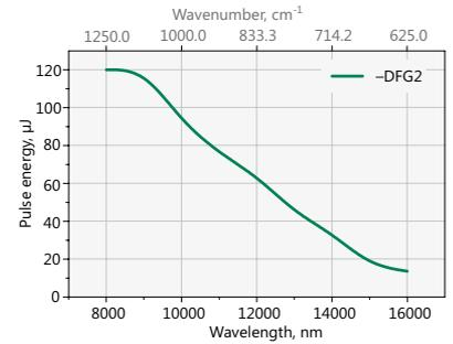
Fig 5. Typical PG501-DFG2 tuning curve in 8000–16000 nm range
