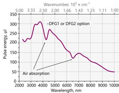
Fig 4. Typical PG501-DFG1 tuning curve in 2300–10000 nm range
