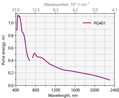
Fig 1. Typical PG401 model tuning curve
