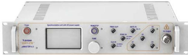
pMaster 4.2 is a timing generator with four output channels used for the full control of operation of high voltage Pockels cells drivers which are built-in in UP2 or MP1 pulse picking units. pMaster 4.2 also has built-in high voltage power supplies for Pockels cells drivers powering.
