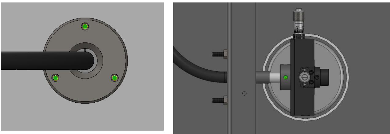
Figure 29: Positions of screws on the feedthrough (L) and retaining screw on the LLG mount (R).
