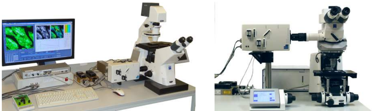
Fig. 1: The DCS-120 system with a Zeiss Axio Observer microscope (left) and Zeiss Axio Examiner (right) .
