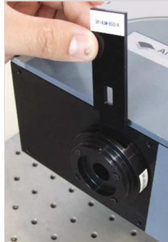
**Step 2:** Place the Adapter (part # **SR1-ASM-8032-B**) in the Slit Holder:
