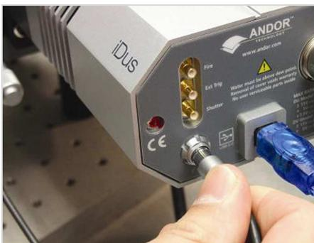
Figure 1: Connecting I<sup>2</sup>C shutter control cable from SR1-SHT-9003 shutter directly to camera
