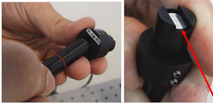
**Step 2:** Tighten the 4-off M3 nylon tipped grub screws:
