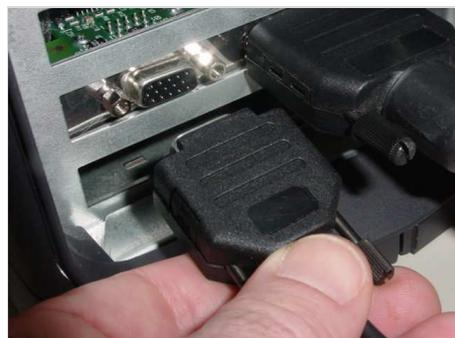
Figure 2: Connecting shutter control cable from SR1-SHT-9004 shutter to PCI card
