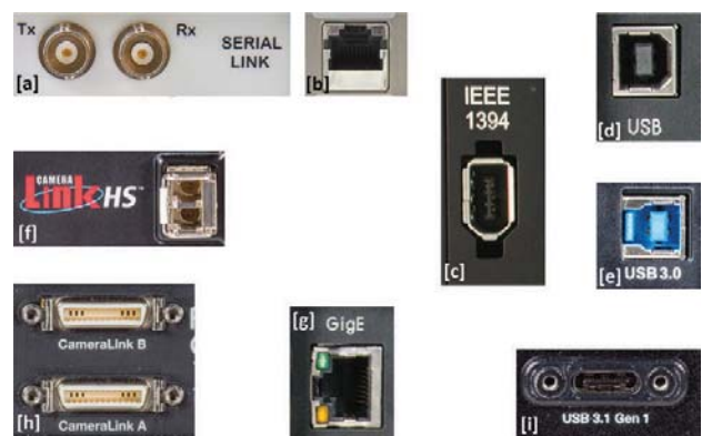
Figure 1: Photos of a variety of image data interface connectors: [a] proprietary highspeed serial data interface based on coaxial cables, [b] proprietary highspeed serial data interface based on LAN cables, [c] IEEE 1394 a “Firewire” interface, [d] USB 2.0 interface (device side), [e] USB 3.0 interface (device side), [f] Camera Link HS interface, [g] Gigabit Ethernet interface, [h] Camera Link Full interface and [i] USB 3.1 Gen 1 interface.
