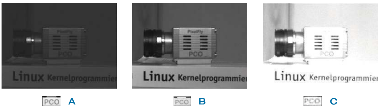
Figure 2: The same series of images with increasing binning from (a) to (c) (like above), only the images with lower resolution have been blown up in size, show the loss in spatial resolution. The detail images showing the letters “PCO” have been further processed in terms of brightness and contrast to elucidate the loss of spatial resolution by binning.
