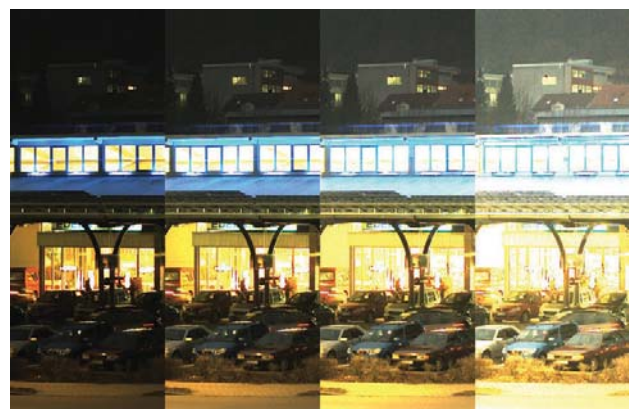
Figure 1: Four extracts of the same night image, which was taken one evening outside the lab of a supermarket in Kelheim using a pco.edge 5.5 color sCMOS camera system. Each image demonstrates how the 16 bit image was scaled to the 8 bit world of the print or the screen, but all versions have been created from the same raw data file. The image on the left side shows a full scale conversion (value 65536 (16 bit max) -> value 256 (8 bit max) and value 0 (16 bit) -> value 0 (8 bit)), while image on the right shows a low scale conversion (value 1024 (16 bit low) -> value 256 (8 bit max) and value 0 (16 bit) -> value 0 (8 bit)). The other images show different conversions in between.
