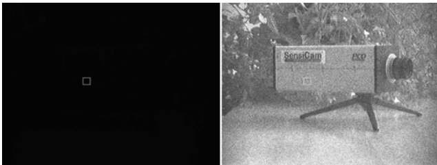
Figure 1 Left image: scaled to full scale 0 - 4095 => 0 - 255 Right image: scaled to minimum - maximum 53 - 75 => 0 - 255 exposure time = 1ms, the white rectangle shows the position and size of the area, which was used to calculate the values for the graph in figure 5.
