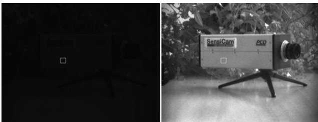
Figure 2 Left image: scaled to full scale 0 - 4095 => 0 - 255 Right image: scaled to minimum - maximum 62 - 190 => 0 - 255 exposure time = 10 ms (for white rectangle see legend figure1)
