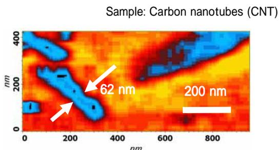
Silver particles distribution on CNT layer. Raman image at CNT G-band line (1593 cm<sup>-1</sup>).
