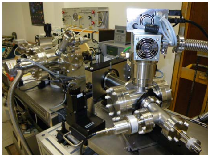
McPherson 642-1 multi-anode soft x-ray calibration light source shown with Model 02 proportional counter and gas flow control system; McPherson, Inc. Model 248/310 soft x-ray grazing incidence spectrometer in foreground.
