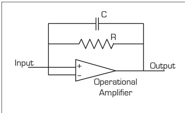
**FIGURE 1. OPERATIONAL AMPLIFIER CIRCUIT FOR MEASURING THE TIME AVERAGE OF A COMPLEX PERIODIC SIGNAL**
