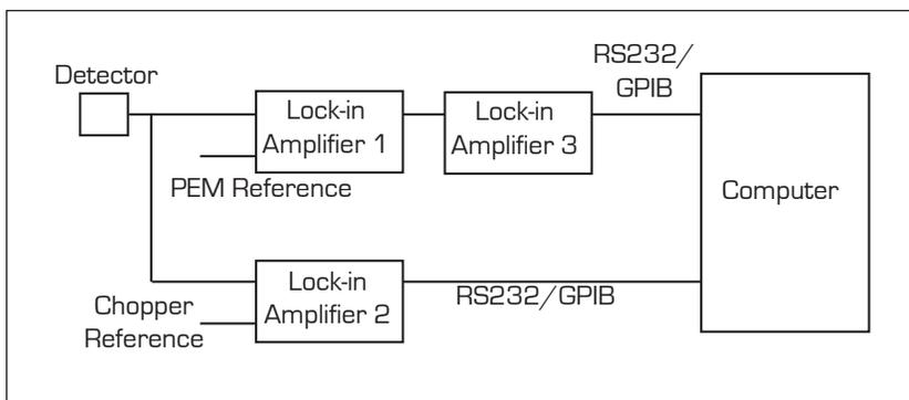
**FIGURE 4. ALTERNATIVE BLOCK DIAGRAM FOR DETECTOR SIGNAL ANALYSIS USING CHOPPING FOR AVERAGE SIGNAL DETECTION**
