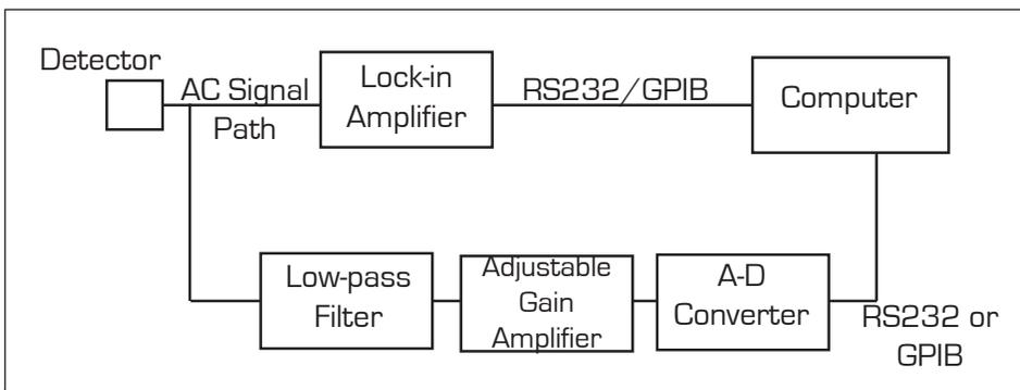
**FIGURE 2. BLOCK DIAGRAM FOR DC-COUPLED AVERAGE SIGNAL DETECTION**
