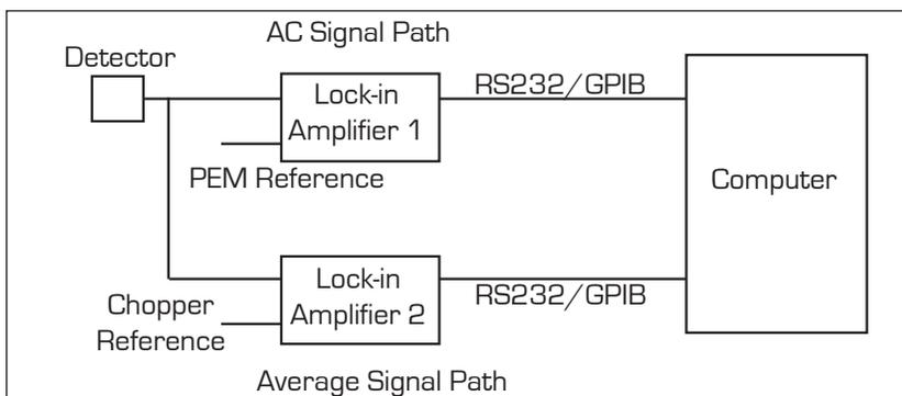
**FIGURE 3. BLOCK DIAGRAM FOR DETECTOR SIGNAL ANALYSIS USING CHOPPING FOR AVERAGE SIGNAL DETECTION**
