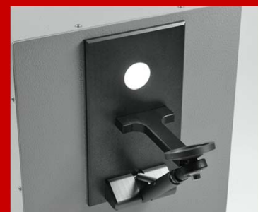
10 mm measurement port of the integration sphere
