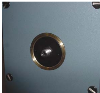
Figure 32: Shutter housing fitted with SMA connector & Slit Disc
