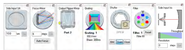
(a) Slit drive: Control the spectrograph slit width - drag blades on icon or type in required slit width
