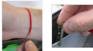
**IMPORTANT NOTE: The ESD strap must be worn at all times when handling the Controller Card.**
