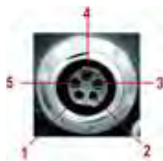
Figure 5: I 2 C connection (facing in) with pinouts
