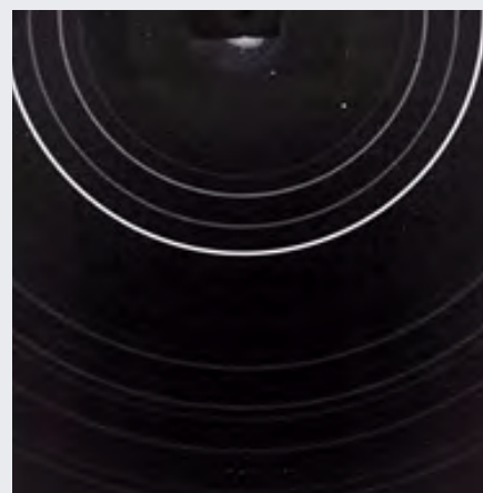
XRD Powder diffraction image obtained with an iKon-L SO. Courtesy of NASA AMES, USA
