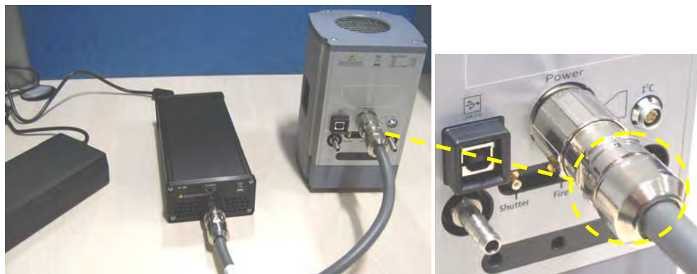
Figure 5: PS30 connected via Power Cable PS40 to camera
