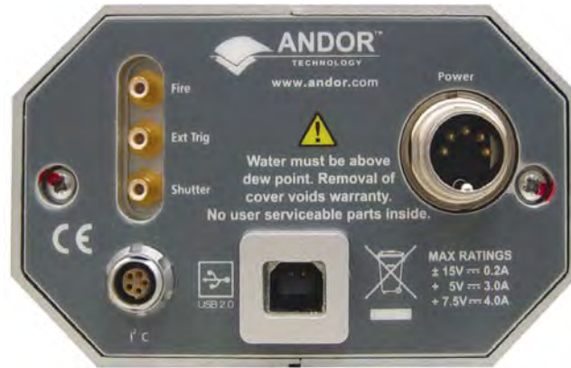
Figure 4: iDus backplate showing connections
