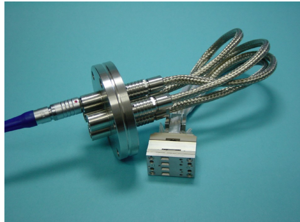
Bolometer with vacuum feedthroughs and low-noise vacuum cable
