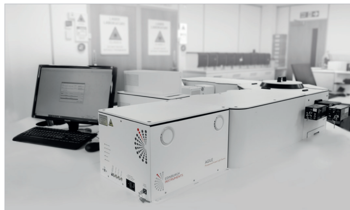
AGILE connected to an FLS1000 Photoluminescence Spectrometer.
