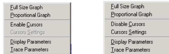
Fig. 62: Select panel for display size, cursor display, and display and trace parameters
