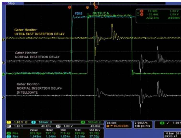
Fire pulse to intensifier opening using DDG
