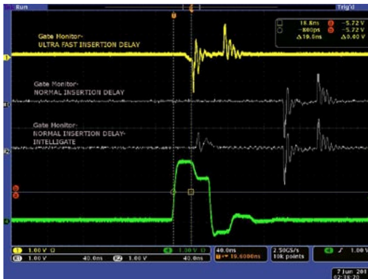
Direct Gate to intensifier opening
