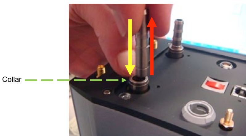
Figure 8: Removal of coolant hose inserts from quick release couplings on camera head
