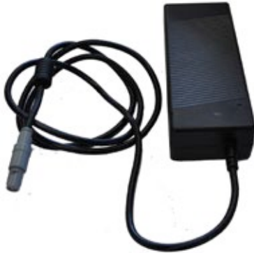
Figure 7: PS-90 power supply for the New iStar
